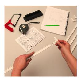
Insert the corners into the frame. You will need a mallet or hammer to tap them into the profile. They are designed to be a tight fit to give you a solid frame but if you are finding the fit too tight you can rub the arms of the corners down lightly with a piece of sand paper.
