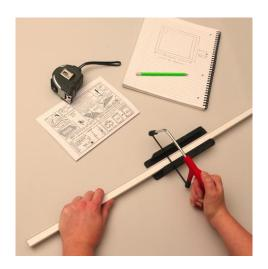
• After double checking your measurements, use a hacksaw and mitre box (if you have one) to cut each of the 4 pieces to the required length.
